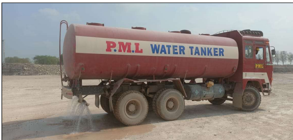
Haul Road water Spraying
